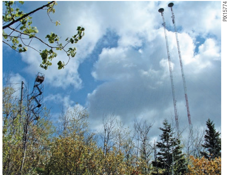
The first anemometer on Mount Maude on the Grand Portage Chippewa reservation in northeast Minnesota was mounted at 20 meters on the fire lookout (left) in January 2004. In January 2007, anemometers were mounted at 30, 50, and 80 meters off the ground on TV towers on Mount Maude (right).
