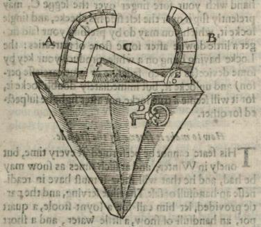
fitted unto it to unlocke it, as may appeare at B. And lastly, let the bows have divers notches filed in them, so the place of the partition when the locke is shut home will be least of all suspected. By this figure and directions you may fit your selfe of such a Locke if so be you are desirous of it.
