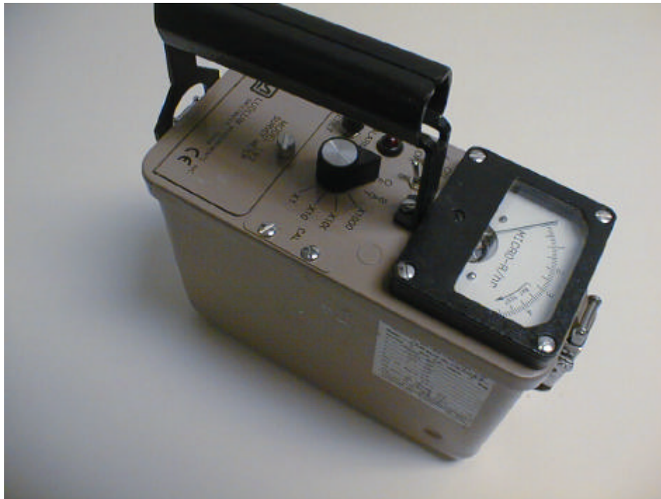
Figure 5- MicroRmeter (Ludlum Measurements, Inc., appendix 1) used to measure gamma activity associated with naturally occurring radioactive materials at an oil and gas production site.
