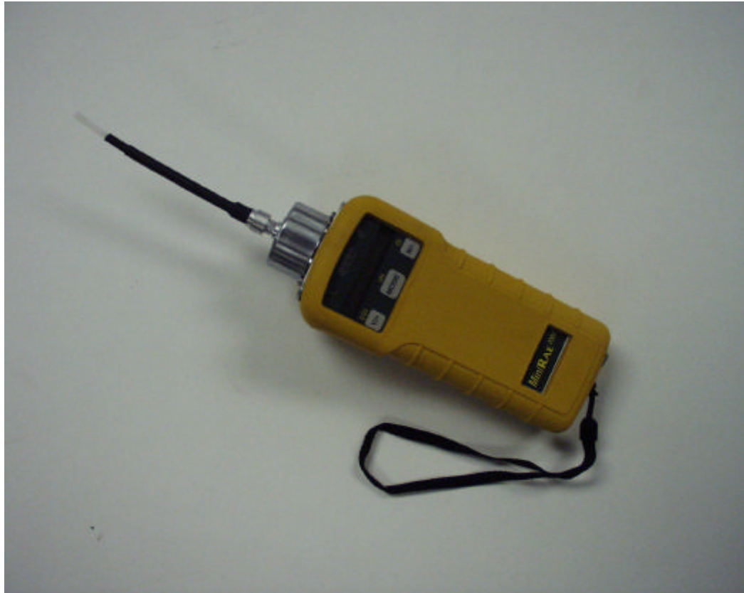
Figure 2- Photoionization detector (RAE Systems, appendix 1) used to determine the concentration of volatile organic carbons in air (either in soil gas in an auger hole or being given off by a soil sample to the headspace of a plastic sample bag).
