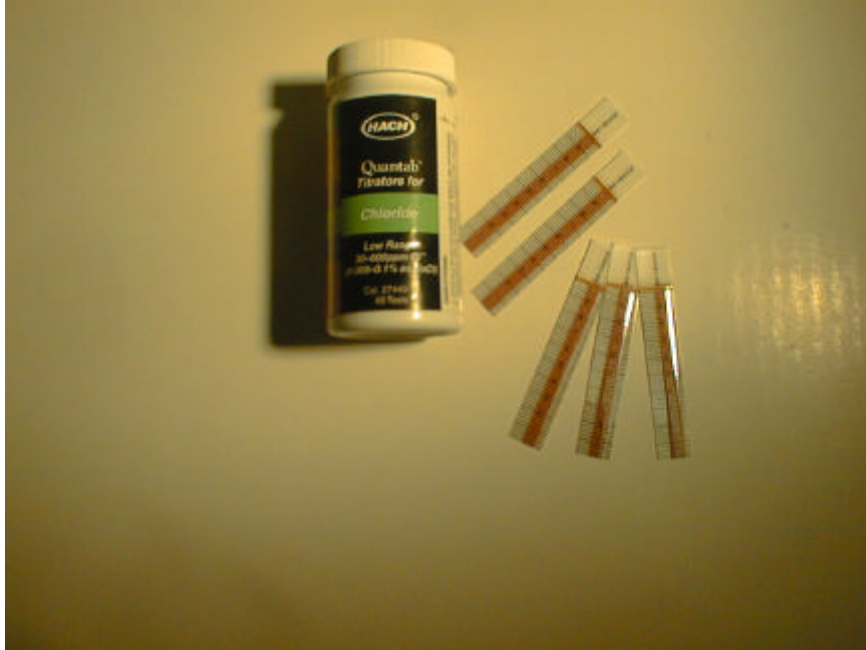
Figure 4- Chloride titration strips (HACH Company, appendix 1) provide measurement of chloride ion concentrations in sampled waters or in soil leachates.
