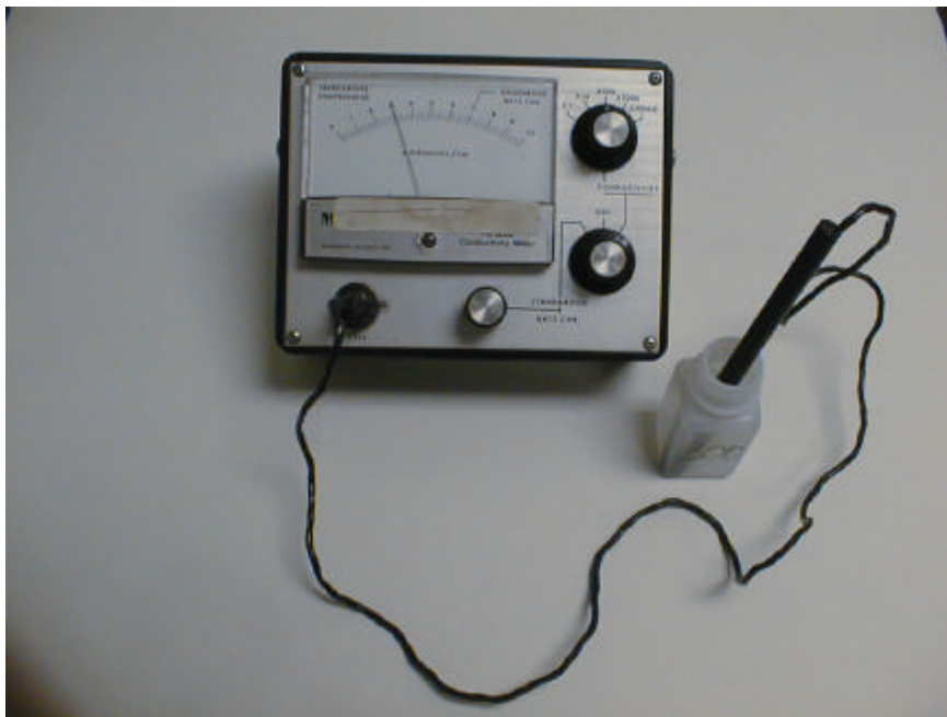
Figure 3- Field conductivity meter (Markson Science, appendix 1) used to determine conductivity of water samples and soil leachates.
