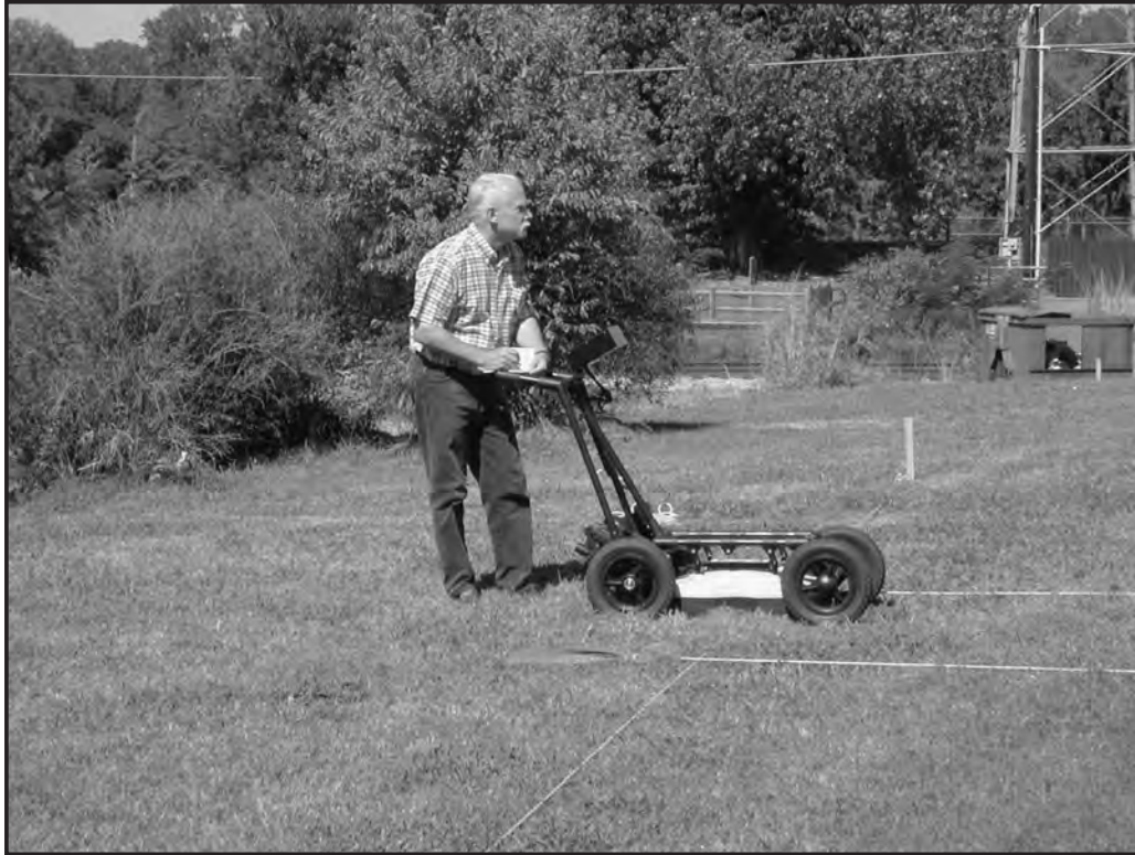
Figure 3. Ground-penetrating radar unit being prepared for use near Bastion 1.
