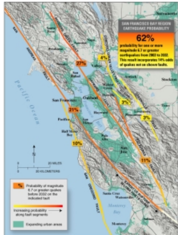
Figure ES.1. Probabilities of one or more major ( M \geq 6.7 ) earthquakes on faults in the San Francisco Bay Region during the coming 30 years. Color indicates the probability that each fault segment will rupture in such a quake.
