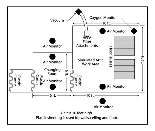
Figure 8: Diagram of Attic Containment System Used in Phase 1 Simple and Complex Simulations of Consumer Use of Attic Vermiculite Insulation
