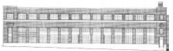
With the proposed glazing system all evidence of the former cargo bay doors is obscured. Modifications to the proposed design such as altering the light pattern to resemble the original door panels as well as adding some solid panels need to be made in order to bring the project into conformance with the Standards.
