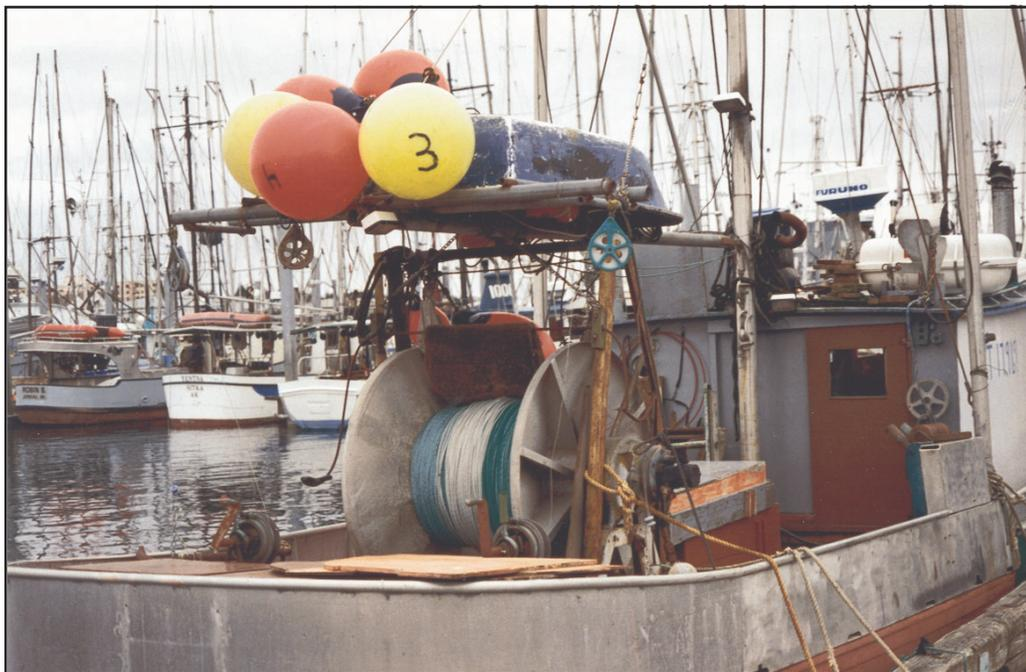
**Photo 3:** A long line commercial fishing vessel
