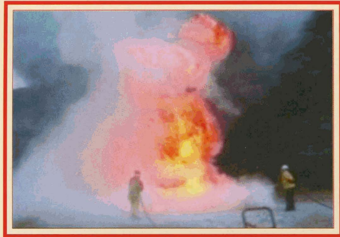
Figure 6. Extinguishing a 400-ft 2 liquid fuel fire
