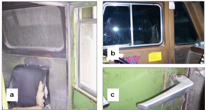
Figure 3. Examples of Old-Style Cab, a) and b) steel interior with older sealants and gaskets, and c) older door handle.
