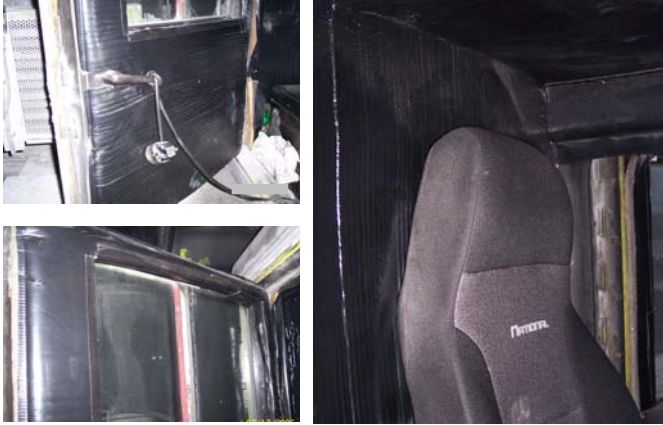
Figure 4. Examples of Retrofitted Cab, foam sound-absorbing material with sealants and gaskets around doors and windows.
