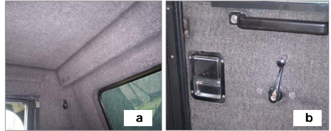
Figure 2. Examples of New-Style Cab, a) full-upholstery and window seals b) newer gaskets, door handles, and window cranks.
