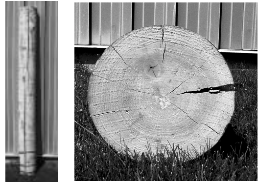
Figures 8. Splits in the Propsetter support typically do not decrease its rated capacity, which is controlled by the wedged section at the bottom of the prop and not the main body of the post.
