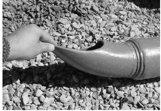
Figure 3. Directional elbow for bulk fill placement.
