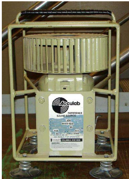
Calibrated noise source for underground testing.
