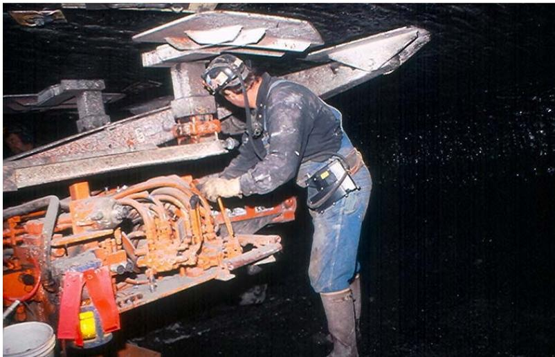
Figure 1. A miner wearing the PDM.
