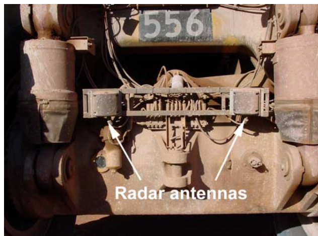
Figure 3. Preview radar system with two antennas.
