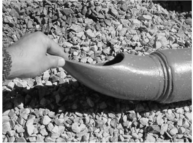
Figure 5. Elbow for bulk fill placement.
