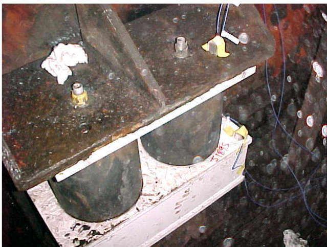
Figure 7. Accelerometers affixed to screen and base at isolator mount locations.
