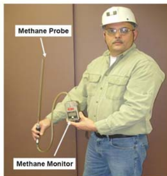
FIGURE 10. PUMP-TYPE METHANE MONITOR AND METHANE PROBE
