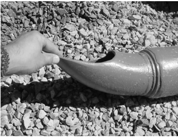
Figure 6. Elbow for bulk fill placement.
