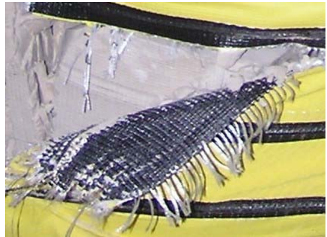
Figure 24. Bag construction showing polyester yarn and waterproof fabric on a section of bag that ripped open during performance testing in NIOSH Mine Roof Simulator.
