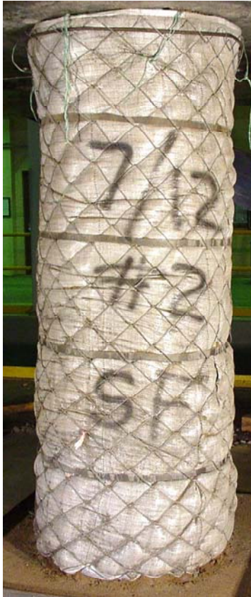
Figure 9. Mesh Pack pumpable support showing laboratory test specimen on left and in mine trials on right (courtesy of Strata Products USA).
