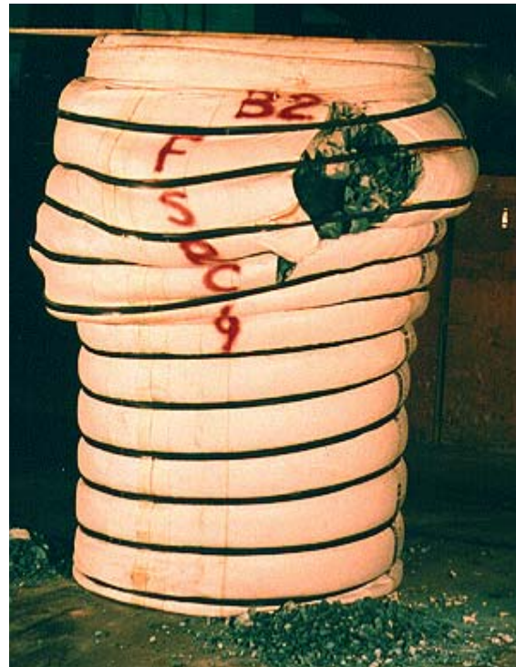
Figure 7. Tekcrib support. Version of this support was first pumpable support installation in longwall tailgate in the U.S. in 1993.
