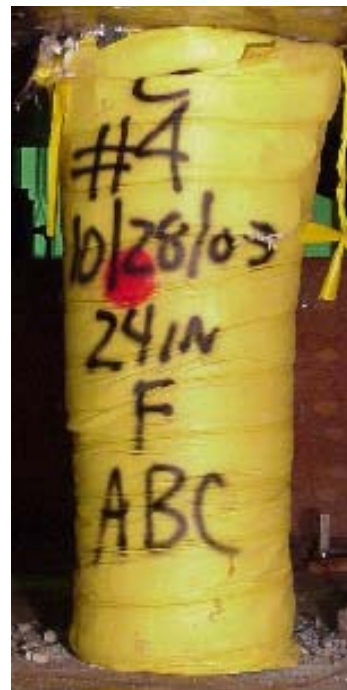
Figure 14. Photo of Tekpak P pumpable support after 6 inches of convergence carrying a load of about 50 tons.
