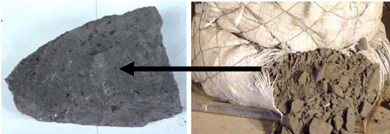
Figure 10. Portland flyash cement product used in Mesh Packs support.
