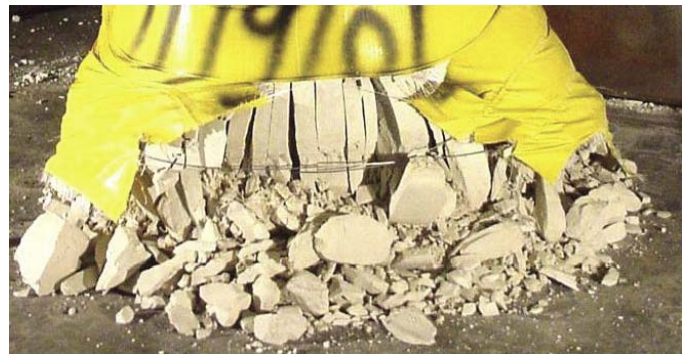
Figure 21. The final product produced from CSA grout is light in color and lightweight.
