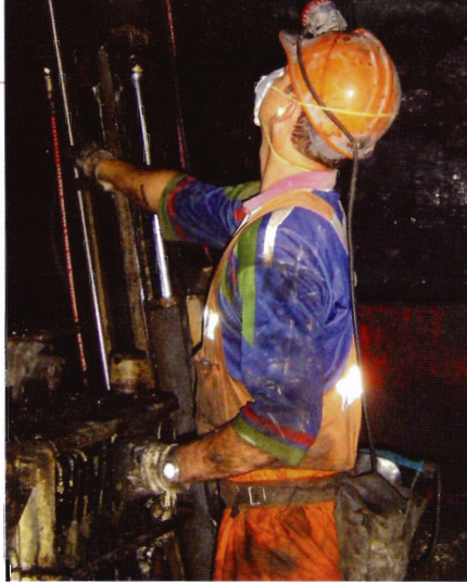
Handling drill steels and bolts away from the body increases the risk of shoulder injuries.
