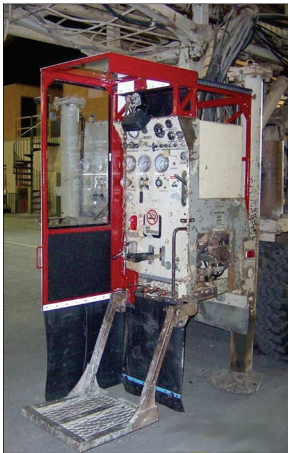
Figure 1. The partial cab is retrofitted to the air rotary drill rig with a steel frame. The cab slides on a heavy duty linear rail that supports the weight of the cab, allows for easy operation, and resists wear.
