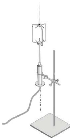
Figure 1. Ultrasonic anemometer on stand.
