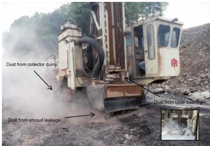
Figure 7. Blasthole drill showing sources of dust emissions.
