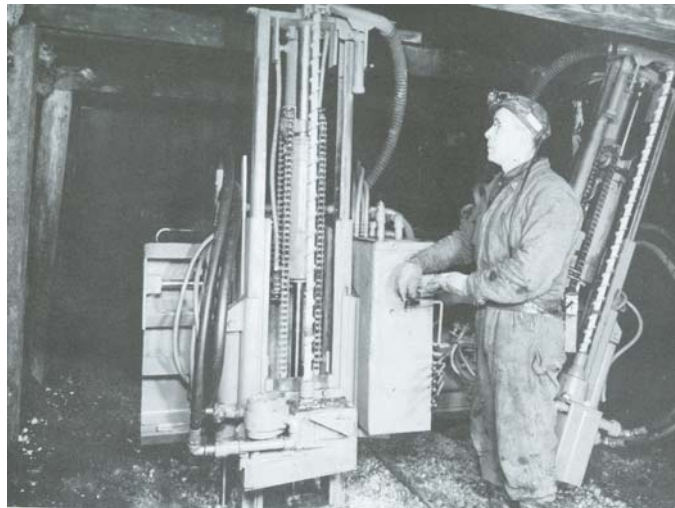
Figure 4. Permissible roof -bolting drill capable of drilling vertical or angle holes.
