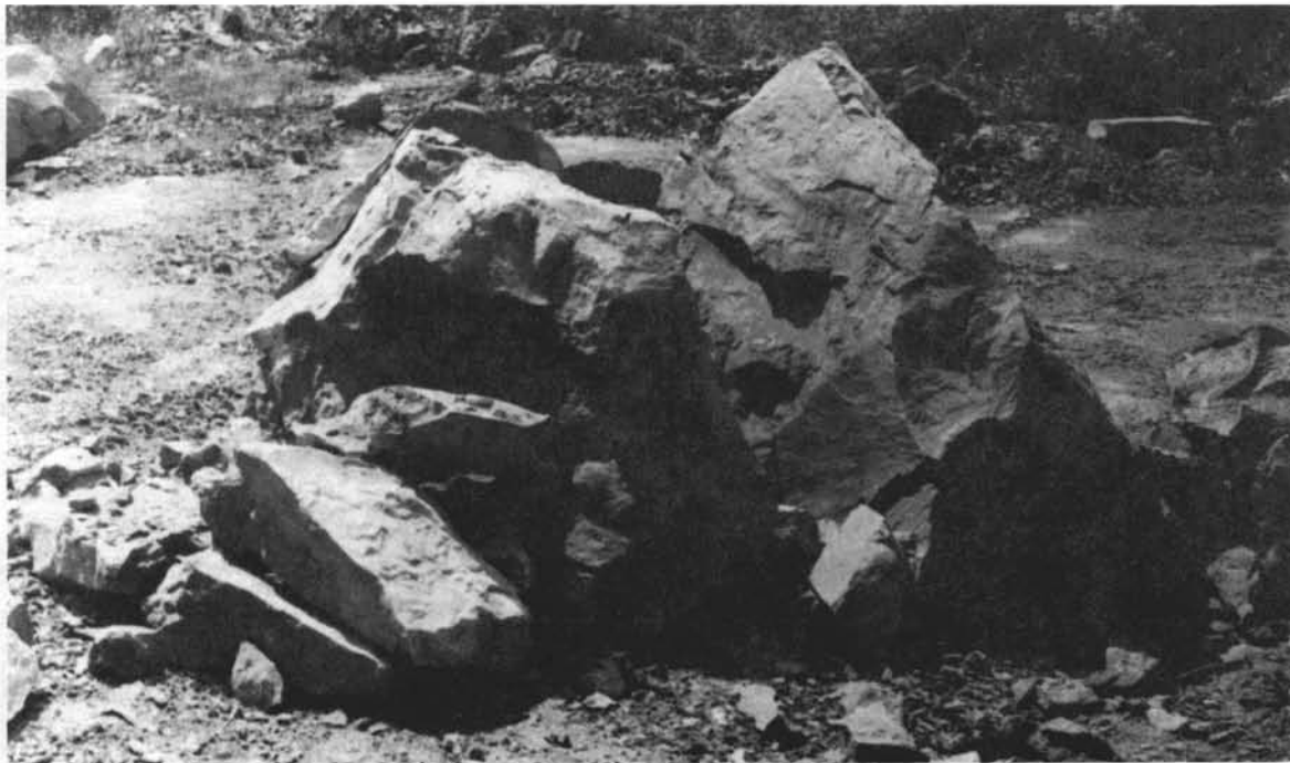
FIGURE 6. - Limestone boulder broken in test 4. Top: Boulder with two nonincendive rock-breaker charges in place. Bottom: Remains of the boulder after firing the charges.
