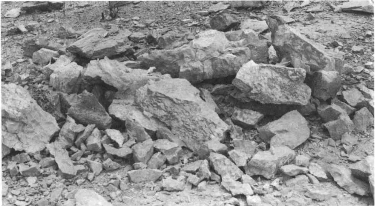
FIGURE 3. - Limestone boulder broken in test 1. Top: Boulder with positioning of nonincendi- dive rock-breaker charge illustrated. Bottom: Remains of boulder after firing the charge.
