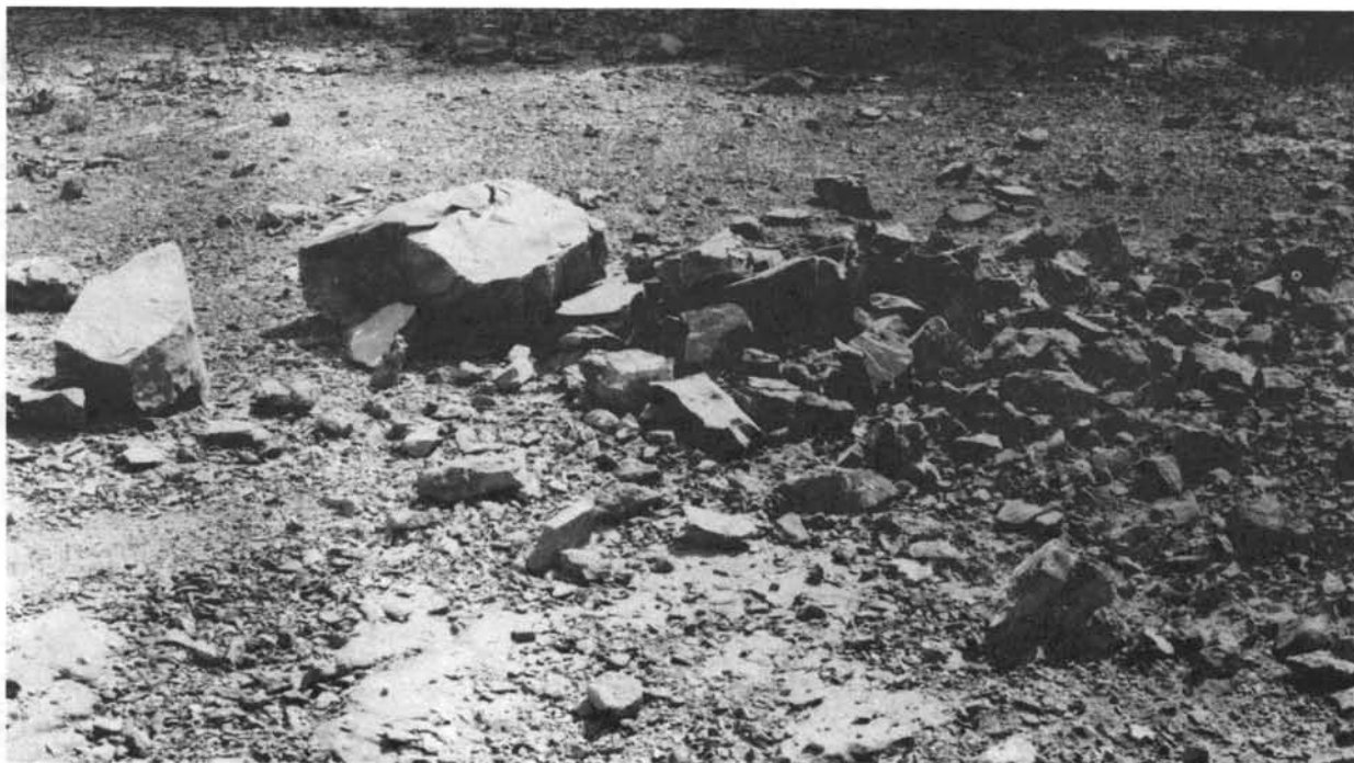
FIGURE 4. - Limestone boulder broken in test 2. Top: Boulder with nonincendive rock-breaker charge in place. Bottom: Remains of boulder after firing the charge.
