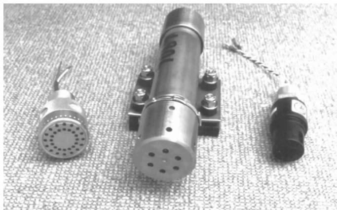
Figure 1. Sensor head for three methanometers.
