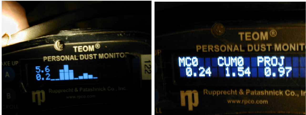
Figure 6.—Basic PDM screen display formats and information presented. Left: graphic format; right: numeric format.
