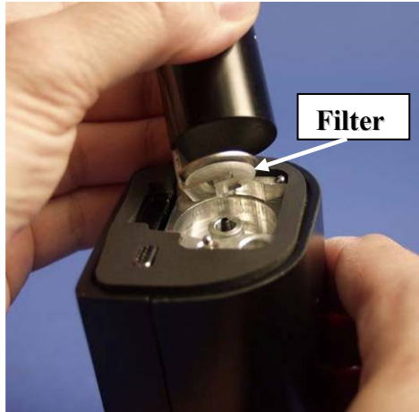
Figure 3.—Technician changing filter on the PDM mass sensor using a custom-supplied filter tool.
