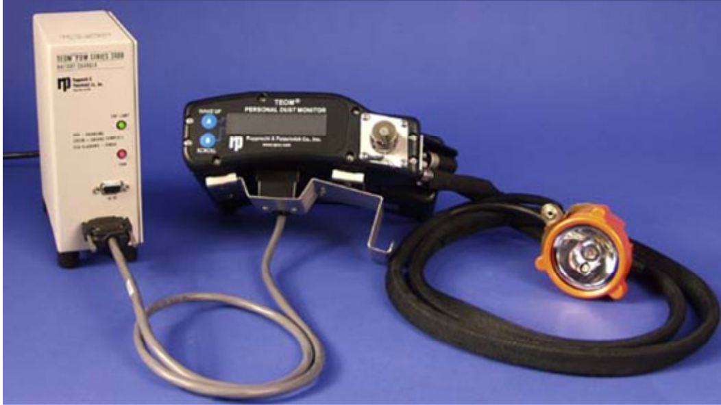
Figure 2.—Precommercial PDM connected to white docking station (left) used for charging and communication with a PC using an RS-232 interface.
