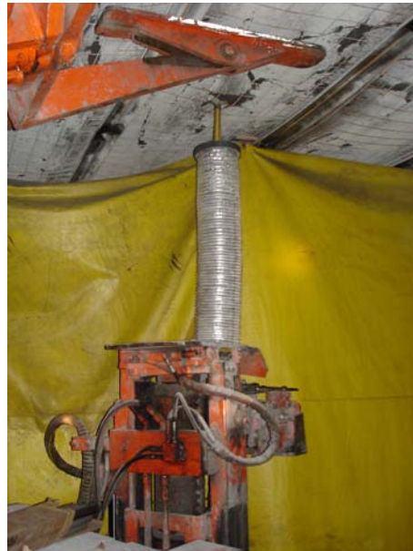
Figure 1: The collapsible drill steel enclosure installed on a roof bolting machine
