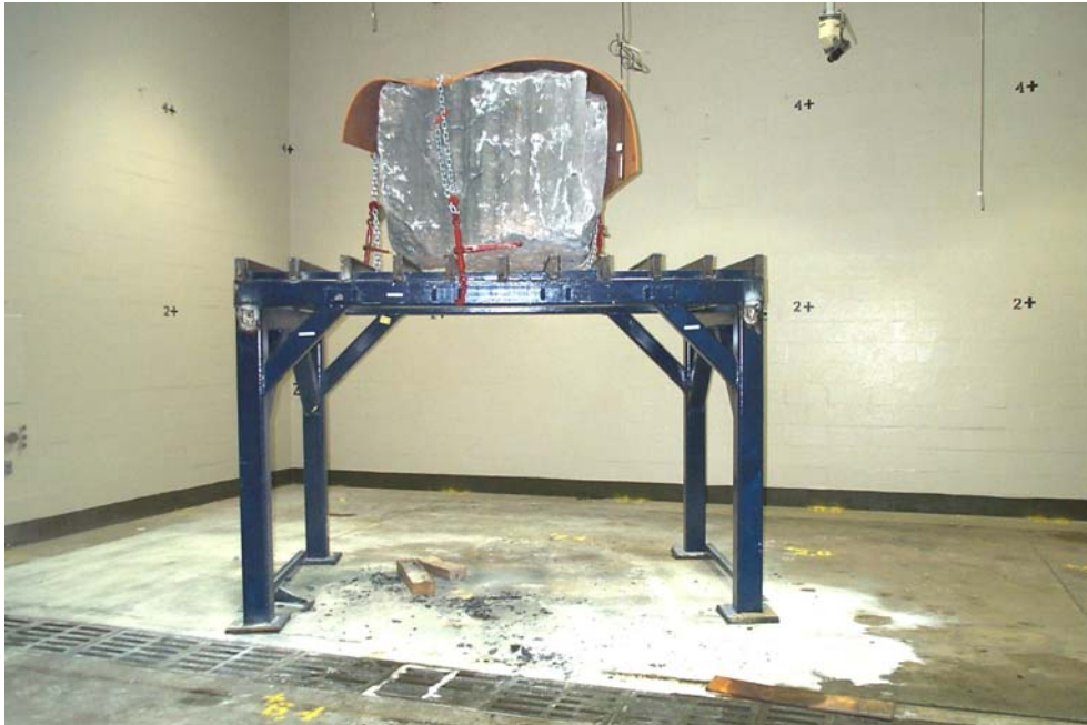
Figure 6: A large steel support stand comprised of rectangular tubes to hold the drilling media.
