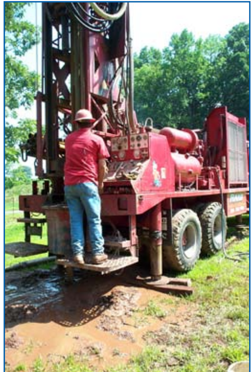
Figure 6. Training younger workers includes more than teaching job–related skills; hazard recognition and health and safety topics should also be discussed. Here a worker operates a rig in muddy conditions that could present a slip/trip hazard.
