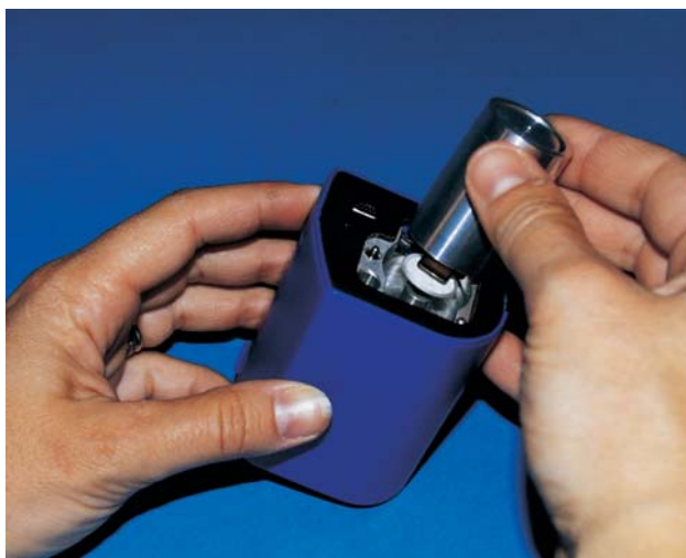
Figure 3-Installing a sample filter in the mass sensor.
