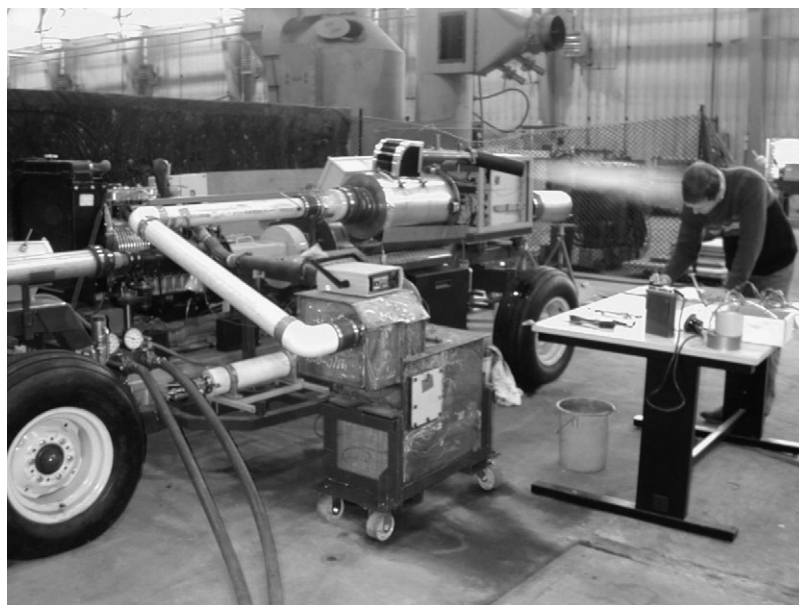
Fig. 2. Mobile engine dynamometer with exhaust of Isuzu C240 engine connected to stainless steel water bath in foreground used for preliminary laboratory testing at NIOSH/PRL.
