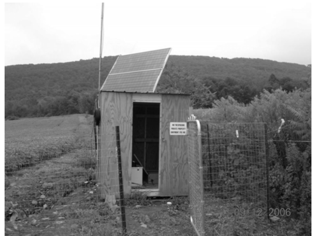
Figure 2. Microseismic data acquisition station at a borehole site.
