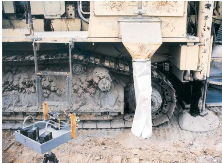
Location of sampling equipment with respect to dust collector dump point.
