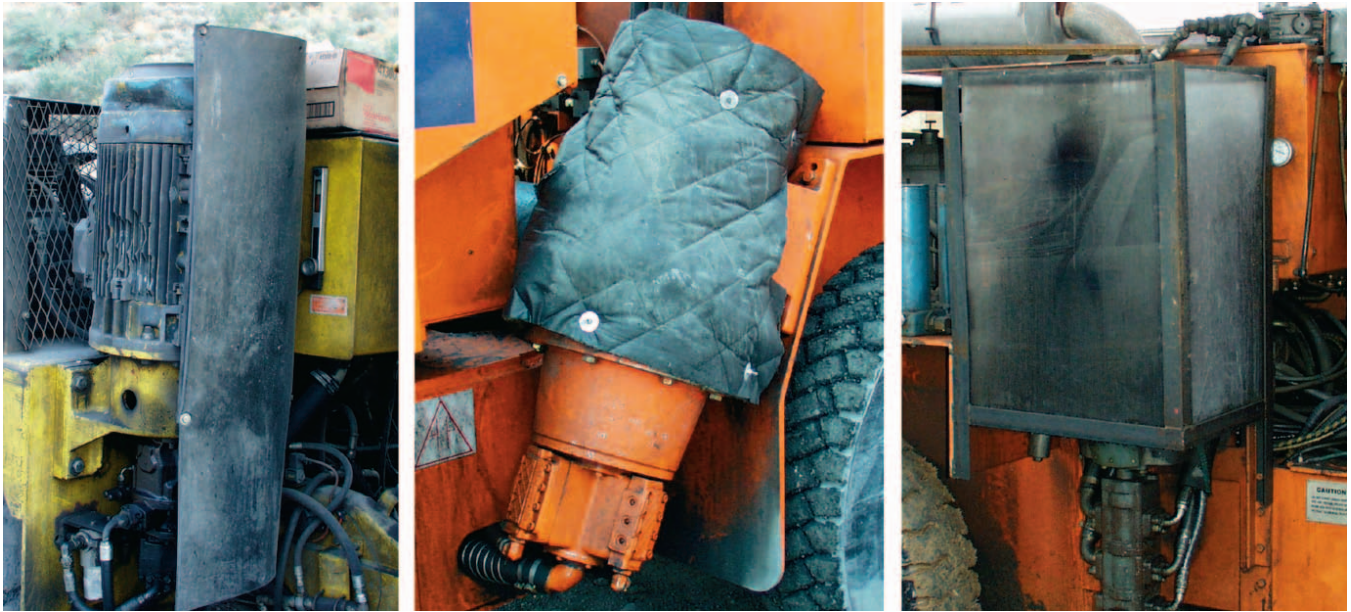
Heavy conveyor belt barrier, fiberglass blanket and Plexiglas motor covers.
