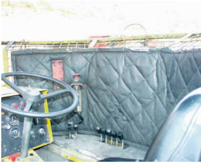
Quilted fiberglass material in the operator's area of Bolter 1.
