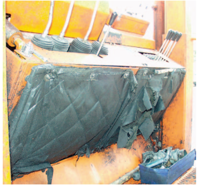
Quilted fiberglass material in the lower front of the operator's area of Bolter 2.
