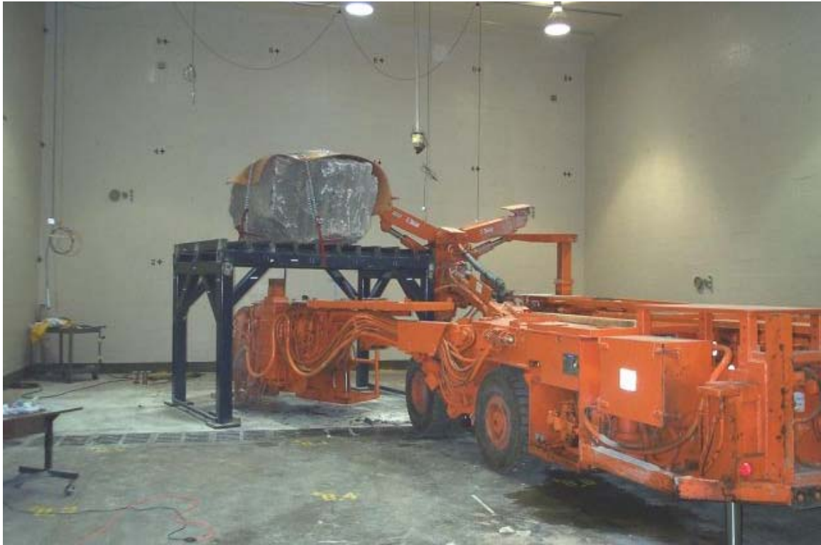
Figure 2. Reverberation Chamber with Roof Bolter During Test Set-up.
