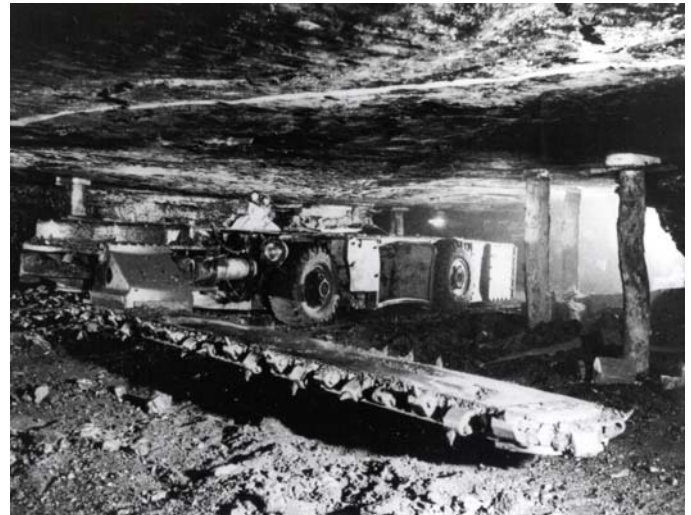
Figure 4. Jay boom cutter used in conventional mining.
