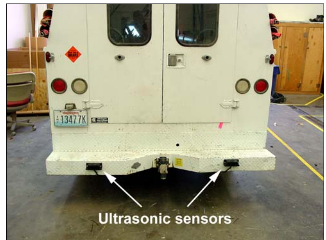
Figure 14.—Hindsight system sensors mounted on pickup.
