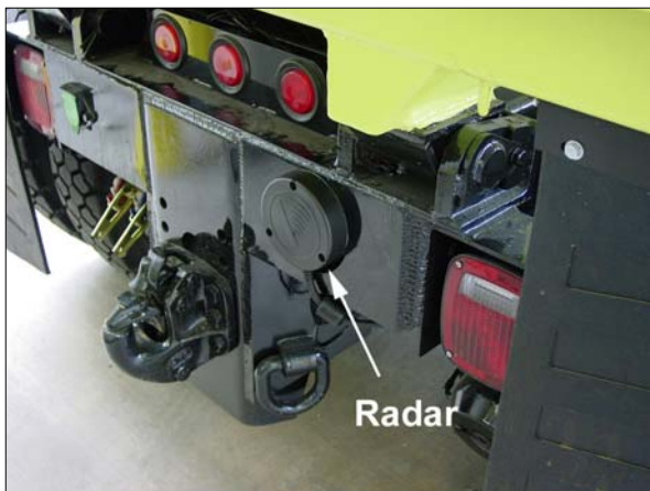
Figure 3.—Preview radar antenna mounted on hitch plate.
