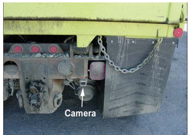
Figure 8.—Intec camera mounted near hitch.
