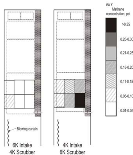
Figure 17. Methane from scrubber exhaust.
