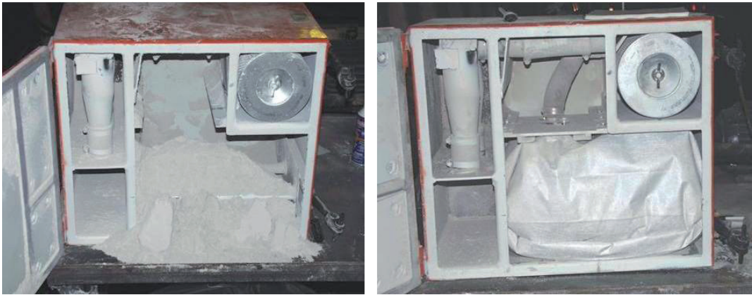
Figure 5. Dust deposited in the collector box (left) and the collector box with bag utilized (right).
