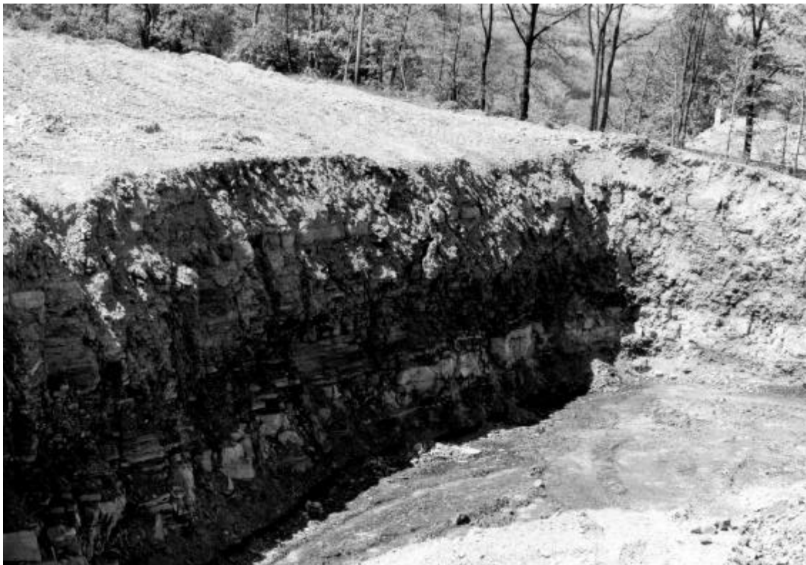
Figure 1.—Blasting in this coal strip mine generated CO that is believed to have poisoned nearby residents.
