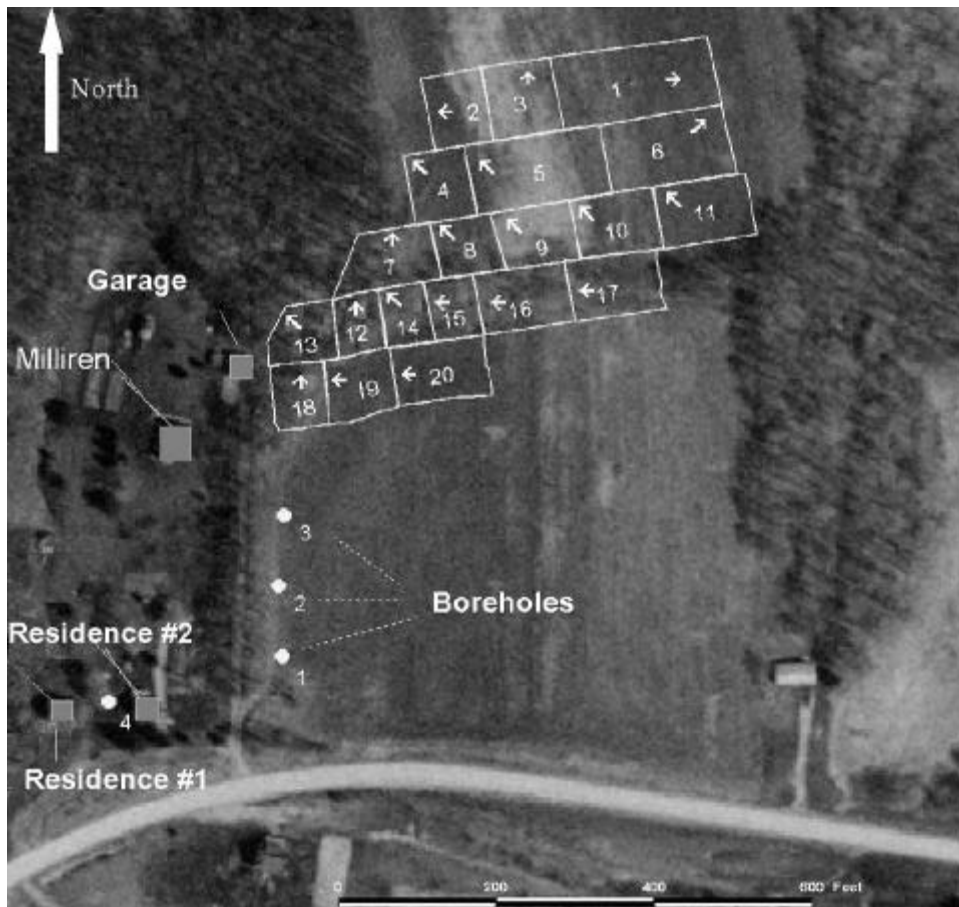
Figure 2.—Map showing blasting at the strip mine and the location of nearby residents. The house labeled "Residence #1" is where the family suffered CO poisoning.
