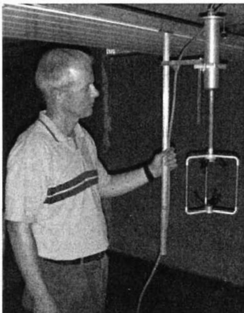
Figure 3 — Three-axis ultrasonic anemometer.
