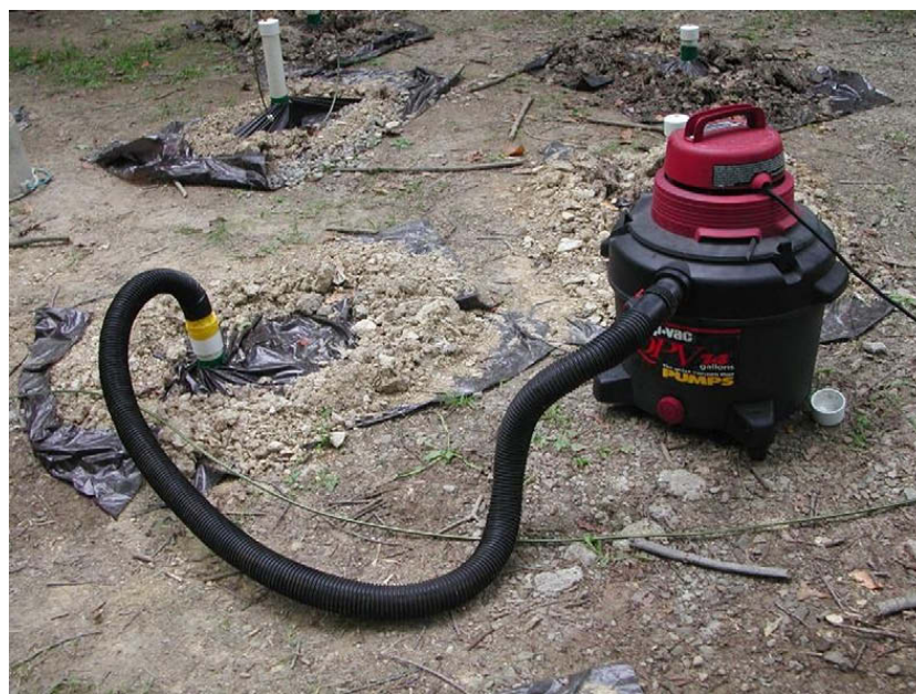
Fig. 3. Negative pressure application using a Shop-Vac.
