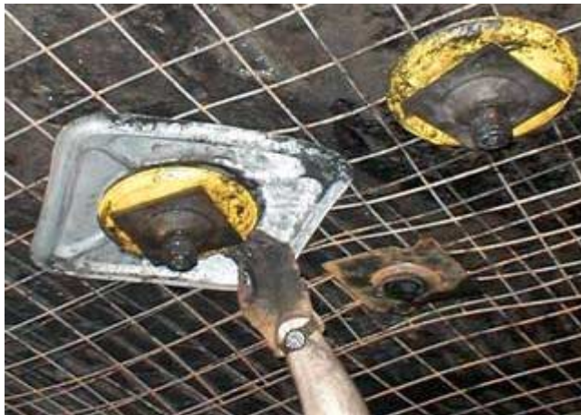
Figure 6. Donut-shaped PSU used to pretension cable bolts.
