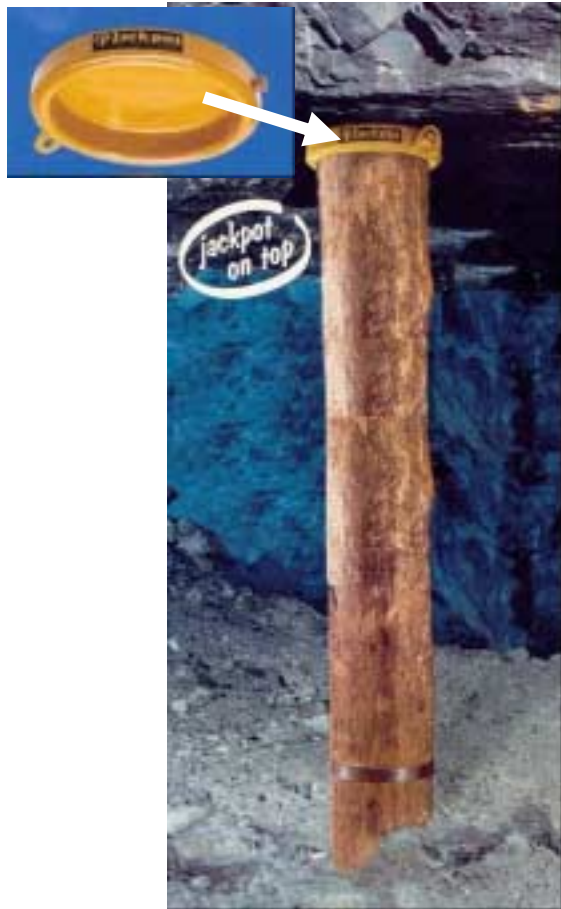
Figure 3. Jackpot prestressing cap on a timber post.
