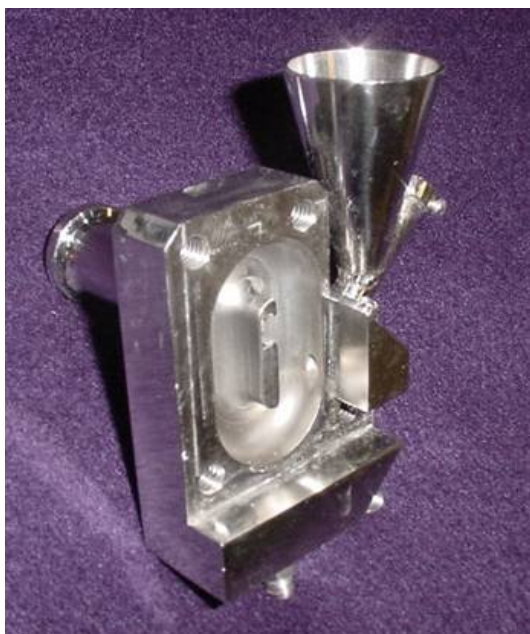
Figure G-3. Jet Mill Used for Processing Dry MS2
