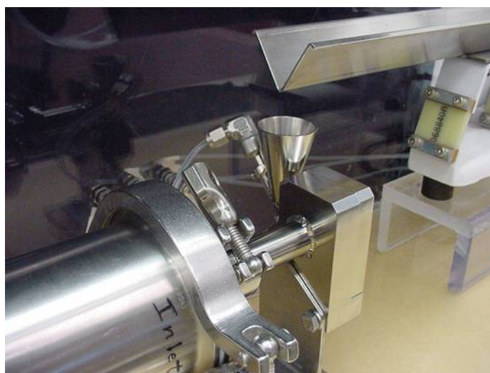
Figure G-4. Jet Mill and Vibrating Feeder Used for Processing Dry MS2
