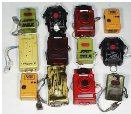
Thermal exposure sensors are embedded in these firefighting devices.
