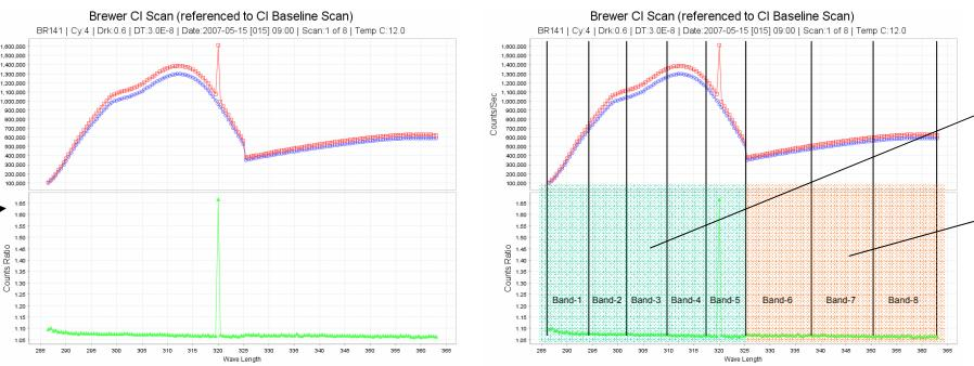
Generating a ratio for CI scans compared to an instrument's baseline reference CI scan.
