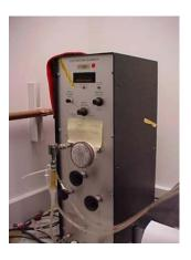
3.1.2. Particle sizing instrument (such as TSI Model 3936 Scanning Mobility Particle Size Spectrometer or equivalent) that is capable of determining submicrometer particles according to count median diameter (CMD).
