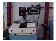
3.1.1. TSI Model 8130 Automated Filter Tester or equivalent instrument. Air flow control accuracy is 2% of full scale. Pressure measurement accuracy is 2% of full scale. Penetrations can be measured to 0.001%, efficiencies to 99.999%.
