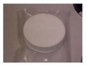
3.1.4. Gelman 102 mm diameter, type A/E glass filters or equivalent high efficiency filters with a 1 micrometer pore size.
