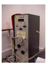
3.1.2. Particle sizing instrument (such as TSI Model 3936 Scanning Mobility Particle Size Spectrometer or equivalent) that is capable of determining submicrometer particles according to count median diameter (CMD).
