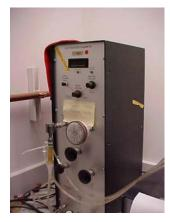
3.1.2. Particle sizing instrument (such as TSI Model 3936 Scanning Mobility Particle Size Spectrometer or equivalent) that is capable of determining submicrometer particles according to count median diameter (CMD).
