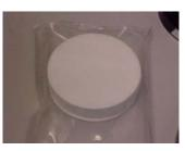
3.1.4. Gelman 102 mm diameter, type A/E glass filters or equivalent high efficiency filters with a 1 micrometer pore size.
